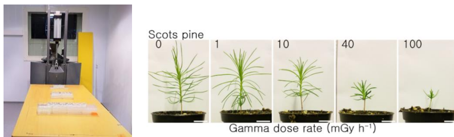
Fig. 1 a) Set-up for exposure of seedlings in Petri dishes to gamma radiation from a ^{60}\text{Co} source under controlled conditions. b) Scots pine seedlings exposed to different gamma radiation dose rates.
