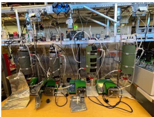
Modified trickle bed reactors for biogas upgrading. Photo: Lu Feng, NIBIO
