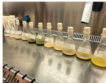
Flask scale experiments of co-culture of cellulolytic strains with oleaginous strains
