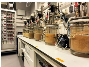
Bioreactor scale-up of SSF using A. corymbifera at 40°C
