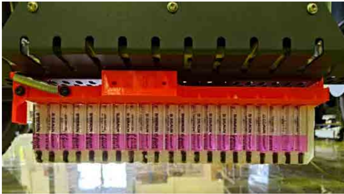
Containers with scale mounted on Kilter AX-1 spray unit. In this test, each container have accumulated the volume from 1000 droplets, proving even distribution (photo: Kilter)
