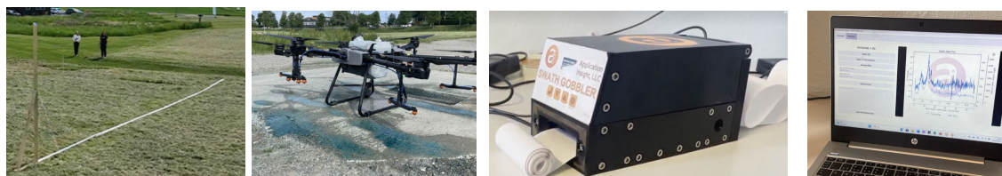
Figure 1: Use of the Gobbler swath analyser; a) set up of paper, b) drone c) paper roll and analyser, d) graph generated on the computer.
