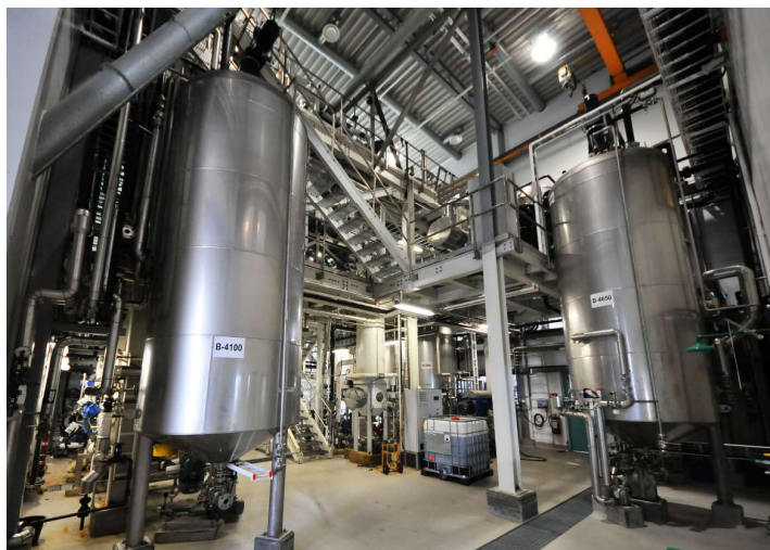
Hydrolysis equipment in Borregaard's biorefinery demo plant used for converting cellulose to sugars.
