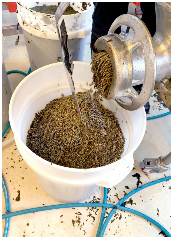
The biomass is thoroughly ground up.
