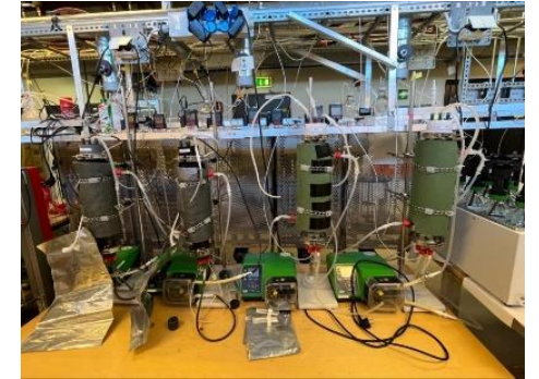
Modified trickle bed reactors for gas upgrading. Photo by NIBIO
